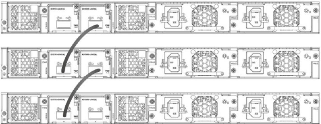
The following figure shows ICX 7450 units connected from 1 X 40-Gbps ports on the rear in a ring stack.
