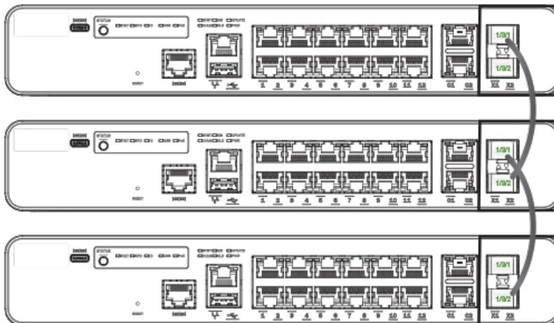
**FIGURE 9** ICX 7150-C12P Stack Ring Topology
