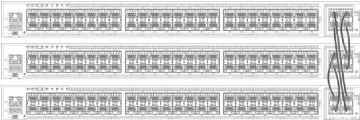
The following figure shows the ICX 7450 connected from the front in a linear stack using stacking trunks.
