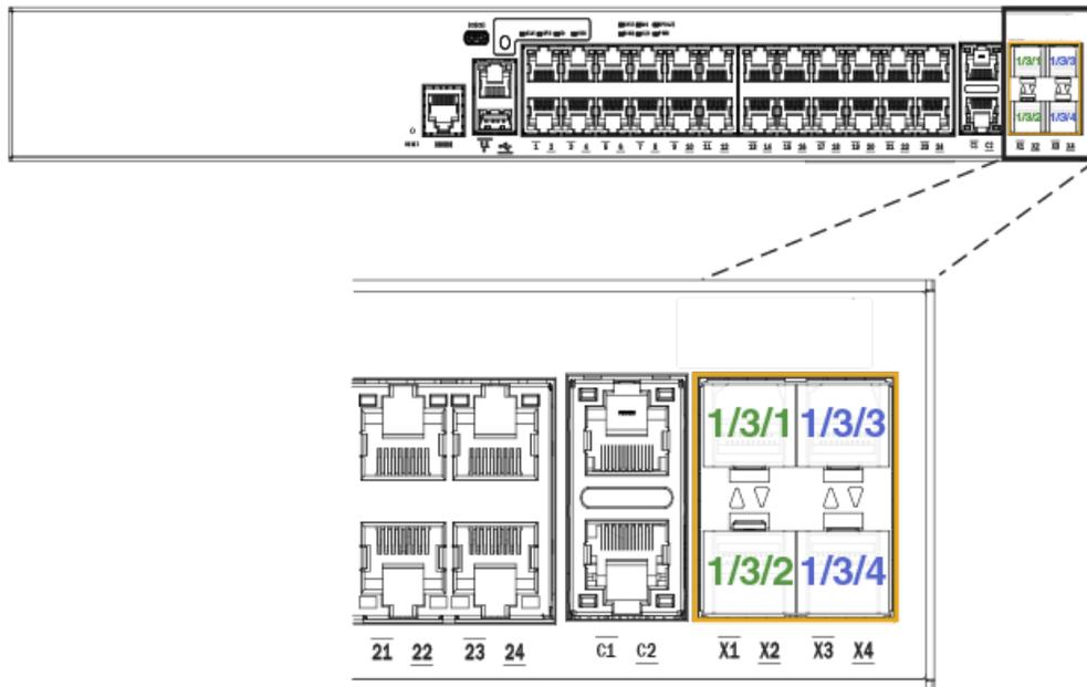
ICX 7150-48, ICX 7150-48P, ICX 7150-48PF, and ICX 7150-24F devices have four stacking ports in the same location on the front panel as ICX 7150 24-port models.
