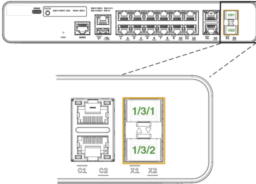
ICX 7150-24 and ICX 7150-24P devices have four stacking ports on the front panel.
