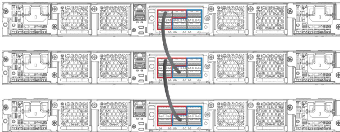
The following figures show ICX 7750 ring stacks from the front and rear panels. Default valid-stack-ports are located on the front panel, but they can be changed to the rear panel using the **stack-port** or **stack-trunk** command.
