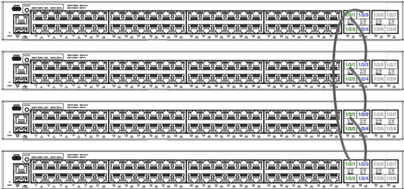
The following figure depicts a two-unit stack linear-topology trunk. All ICX 7150 models except for ICX 7150-C10ZP and ICX 7150-12C devices support this type of trunk, which improves redundancy and bandwidth. For more information, refer to [Support for Two-unit Stack Linear-topology Trunks](#) on page 33.
