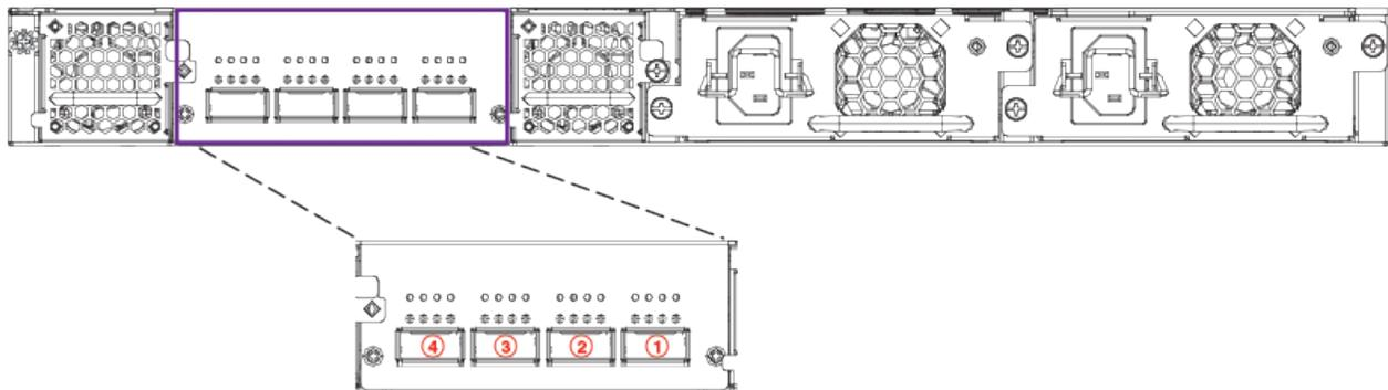
The rear module is fixed, and its ports can be configured for stacking or uplink. By default, the rear module supports 100-Gbps stacking on ports 1 and 2 (1/3/1 and 1/3/2). When 100-Gbps stacking is enabled, ports 3 and 4 are not used. Stacking trunks are not supported on 100-Gbps connections in a stack that contains more than two units. However, a 100-Gbps linear-topology trunk (ports 1/3/1 to 1/3/2) is supported in a two-unit stack.
