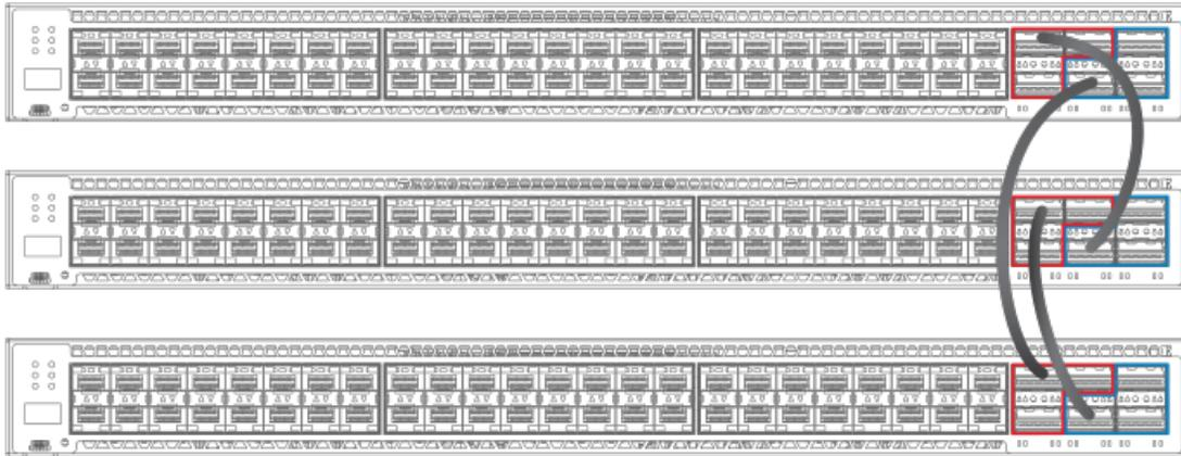
FIGURE 43 ICX 7750 Ring Stack from Rear Panel
