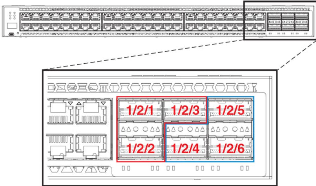
FIGURE 39 ICX 7750-26Q Front Panel Stacking Ports
