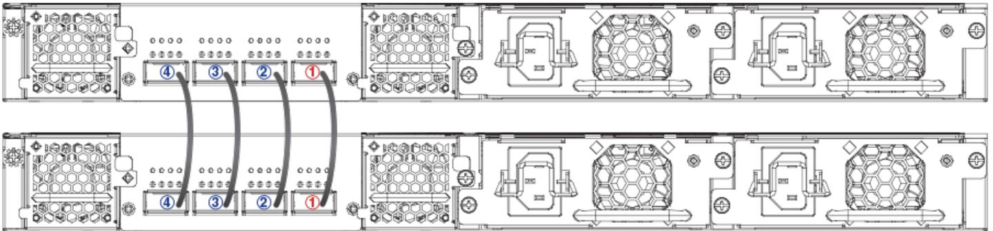
**FIGURE 37** ICX 7650-48ZP Two-unit Stack Linear-topology Trunk (100 Gbps)
